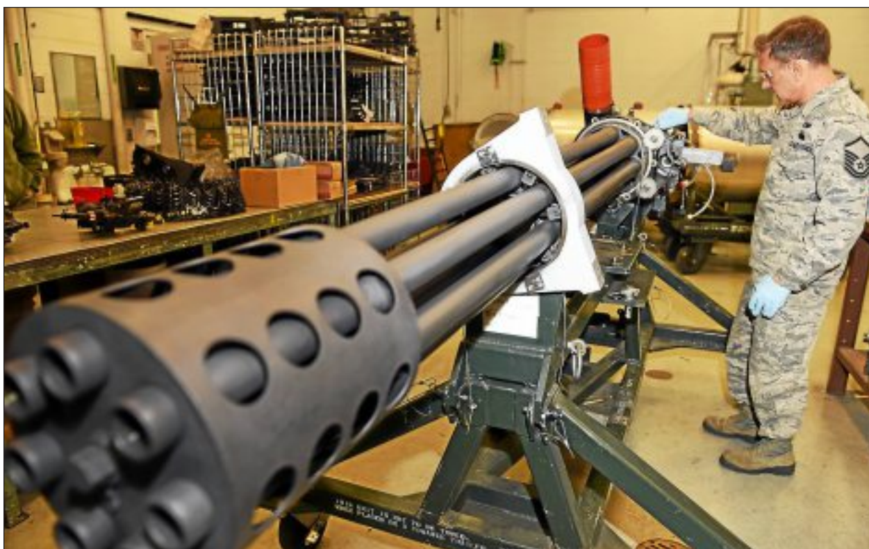
Master Sgt. Thomas Barjaktarovich of the 127th Maintenance Group inspects the 30mm GAU-8 Avenger Gatling gun from an A-10 Thunderbolt II of the 107th Fighter Squadron, at Selfridge Air National Guard Base, Mich., Feb. 5, 2017. The GAU-8 Avenger requires an in depth inspection every 36 months.
