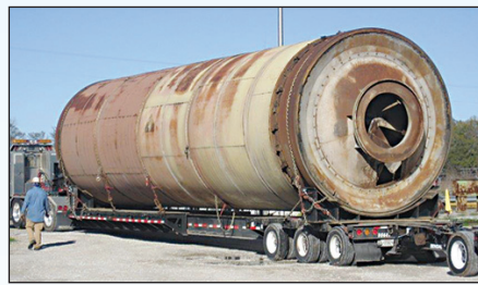
12' x 48' MEC Triple Pass Drum Dryer
