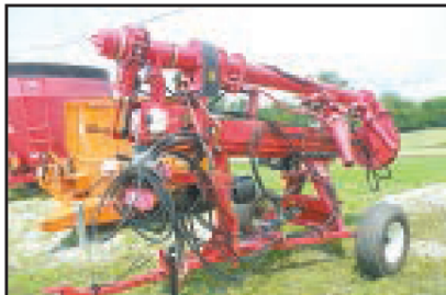
Jamesway 8"x8' Under Floor Pit Pump, Trailer Mounted, (2) Agitation Nozzles w/Hyd. Gate Valve. . . . . In Stock
