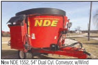
New NDE 1552, 54" Dual Cyl. Conveyor, w/Wind Gds., Full Set Of Knives, 640XL WeighTronics Scale, LED Rd. Lights, Laddery Rubber Top, "New" Redesigned Auger, "Pushes Less Hay Out Over The Top"
