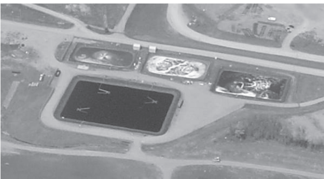
Aerial view of the four Leachate Treatment Ponds at the Crow Wing County Landfill. The treatment ponds are aerated to promote metals precipitation and volatilization of organic contaminants. The ponds are operated in series. The circulating water in the landfill system helps break down trash five times faster.
