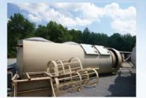
In Stock! Used/Reconditioned Baghouses, such as this Torit 276RF 12—complete with rotary airlock & support steel with capacities from 5,000 CFM to 70,000 CFM depending on requirements. We stock a wide variety of replacement parts for baghouses: filter bags, cleaning head blowers & components, level detectors, rotary airlock speed reducers & drive components.
