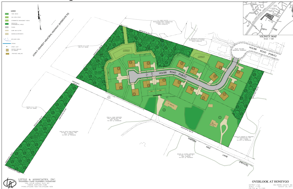
The new development would have access off Holter Road rather than Thirteen Mile Lane, which is a private road. Another piece on the far side of Thirteen Mile Lane would be designated for forest conservation. Image courtesy of Little & Associates, Inc.
