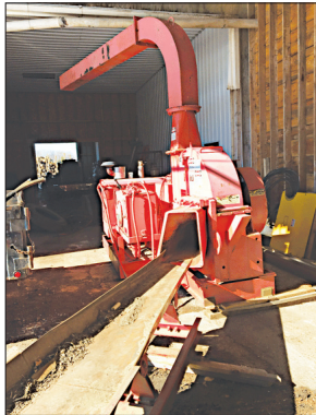
Morbark 48" Chipper, with vibrating feed deck and chute
