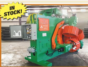
Rebuilt 30" Cambio Debarker Lindsay Air Tension System, hyd. drive, air panel, heavy duty cylinders & feed rolls.
