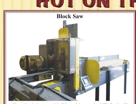
From the designers and builders of the popular M2L Stacker/Unscrambler, the TS300 Stacker and the Center Cut Saw comes the New AIT Block Saw. This new block saw, manufactured by Automated Industrial Technologies and sold exclusively by Pallet Machinery Group, cuts boards, blocks and cants at a rate of up to 2,000 cuts per hour. This production, combined with its high reliability and low maintenance, gives you everything you need in a block saw. No pallet operation should be without it!
