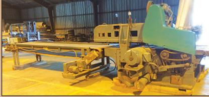
Oliver Strat-o-Planer 1972 late model! Has long infeed belt, spiral carbide heads top /bottom, 36" cut, all electrical included. 30HP to 50 HP. Ready to ship. Weighs almost 18,000 lbs. \$17,5000 for complete system.
