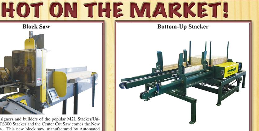
Stack boards at up to 20 layers per minute with Pendu's new 4700B High Speed Bottom-Up Stacker! The bottom-up feed design is lower to the ground than an over the top stacker for easier access to the stick placer and the infeed. The 4700B can handle material from 24 inches to 72 inches long, 1 1/2 inches to 5 1/2 inches wide, and 3/8 inches to 2 inches thick. The stacker can be used with or without an optional pit.
