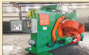
Rebuilt 30" Cambio Debarker Lindsay Air Tension System, hyd. drive, air panel, heavy duty cylinders & feed rolls
