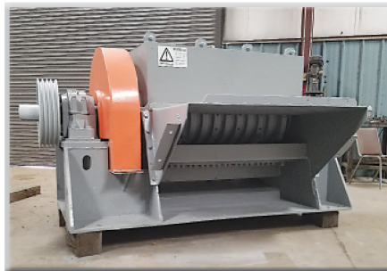
Montgomery Horizontal Hog 9'x 50' feed opening
