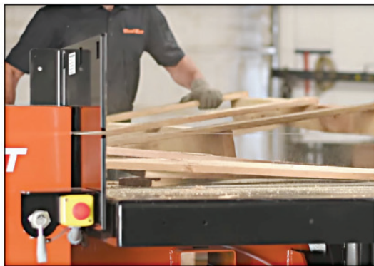
Adjustable table height with 5 1/4" travel
