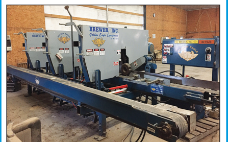
Brewer 3 HD Bandsaw w/Return & Electric Panel
