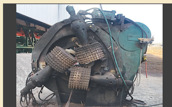
26" Cambio Debarker w/hydraulic drive to include power unit. Infeed also available. All is in good working order
