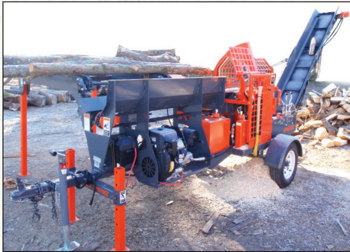
Model 1610EZ Joystick control, gas or diesel, live deck or log lift, ultra mobile with integrated conveyor.
