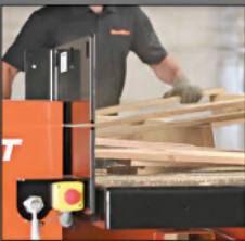
Adjustable table height with 5 1/4" travel
