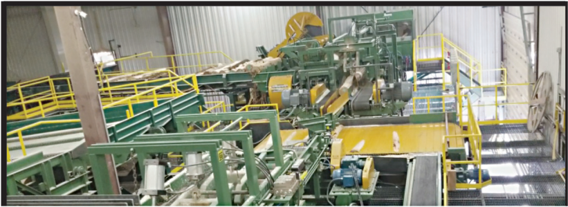
TANDEM SCRAGG WITH TWO HUSK FRAMES A GREAT OPTION TO MAKE LARGE CANTS TO INCREASE YOUR PRODUCTION
