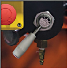
Pneumatic hand valve moves table up and down
