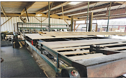
Morris 8 x 16 Green Lumber Stacker with USNR Auto Stick Laying Mechanism
