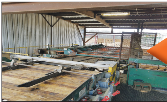
Morris 8 x 16 Green Lumber Stacker with USNR Auto Stick Laying Mechanism
