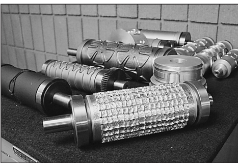
Custom made die-cutting tools are used to create impressions and shapes.
