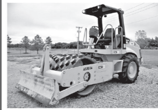
• Sheepsfoot for compaction
