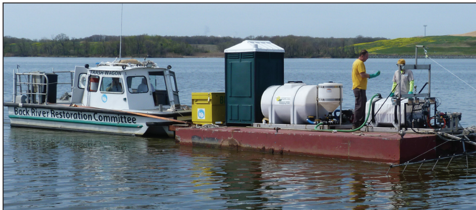
The BRRC volunteered the use of their "Trash Wagon" boat to push the larvacide treatment apparatus. The Bti slurry is injected on the bottom via the boom at the front.
