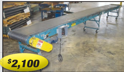
Slider Bed Belt Conveyor 20" x 21' Mounted on legs with casters. 1/2 HP motor with variable speed control.
