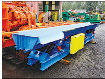
Mill Power Vibrating Conveyor
