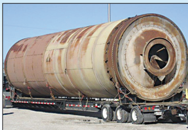
12' x 48' MEC Triple Pass Drum Dryer
