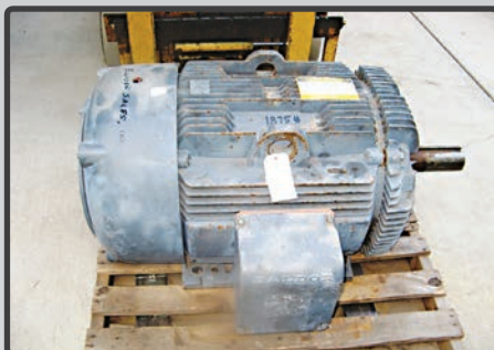
Baldor 150hp 1185rpm TEFC, 10302.01
