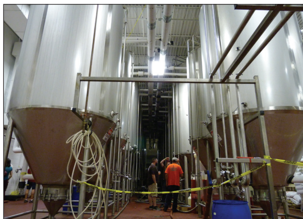
The brewery in Rosedale has 32 fermenting tanks which each hold about 180 barrels of beer at a time. That is equivalent to about 360 kegs or 2,400 cases of beer.
